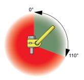
The DLP can only be loaded from 0 - 110 degrees. Rotation around bolt axis when loaded at 0 -15 degrees is not allowed.
